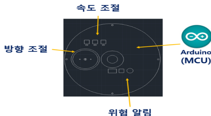
Figure 6 Control part drawing and implementation
